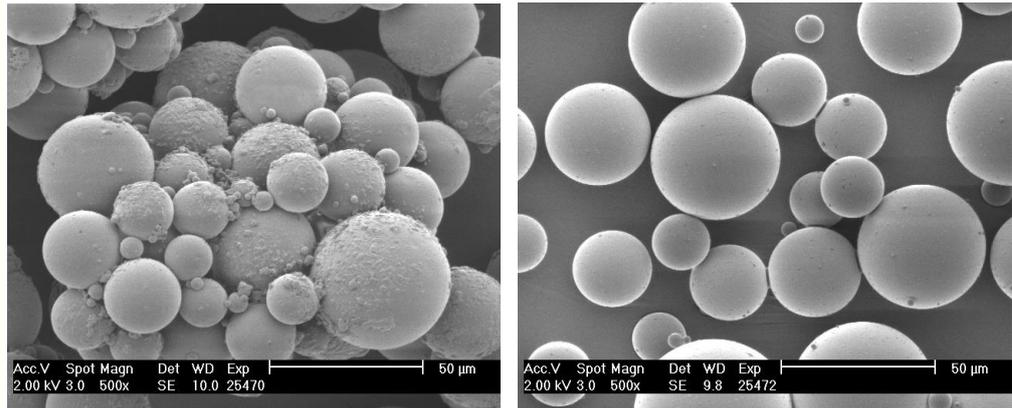
*Fig. 2: Comparison of powders of different tendency to agglomeration.*
