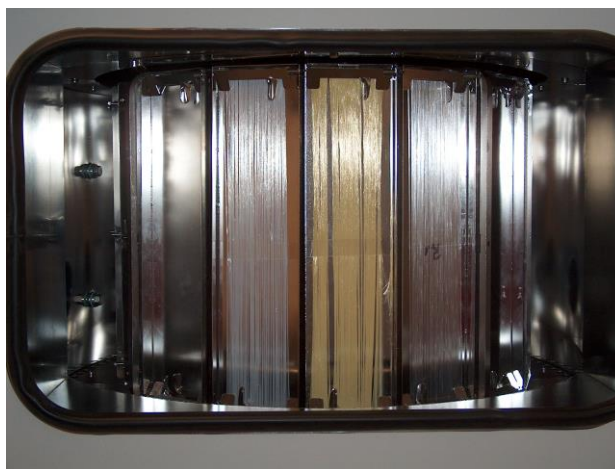
Fig. 2: Xenotest Beta – detailed view on sample carousel with vertically mounted samples.
