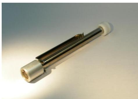
*Fig. 1:* Passive sampler.
