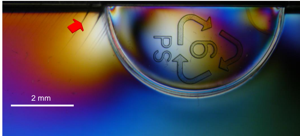
Fig. 3: Incipient stress-corrosion cracking by alcohol.
