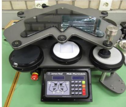
In this test, the fixed flat sample is exposed to a rubbing fabric under defined parameters (pressure, kind of movement, frequency, medium) over a defined period of time.
