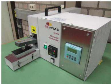
In this test, a movable arm equipped with a rubbing fabric rubs with defined force and number of strokes over the fixed sample. The rubbing fabric can also be charged with media like water to simulate media effects this way.
